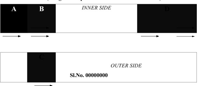
3. Now, there will be an important change in the method of folding the Blue Paper Seal. After fixing the Blue Paper Seal in the slot provided in the windows of the Inner Door covering the Result Buttons, the inner door as well as outer door above the Result Section shall be closed. While doing so, the loose ends of the Blue Paper Seal should be allowed to protrude outside from both the sides of the outer door above the Result Section.
