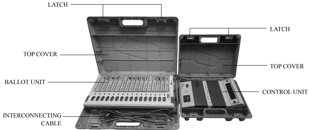
FIG. 1 (A) BU, CU Carrying Cases (open condition)
