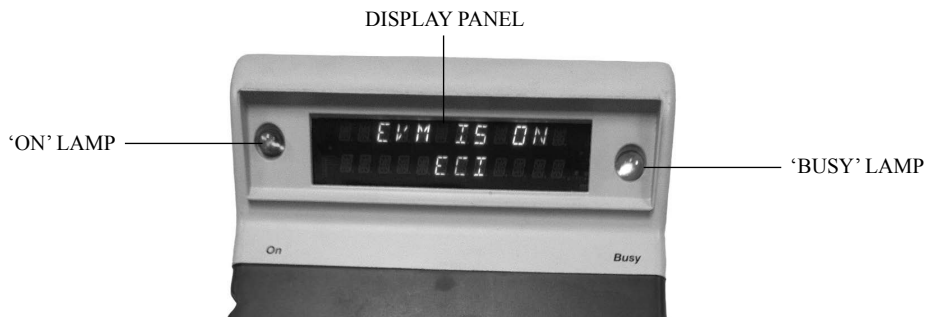
FIG. 13 View of Display Section
