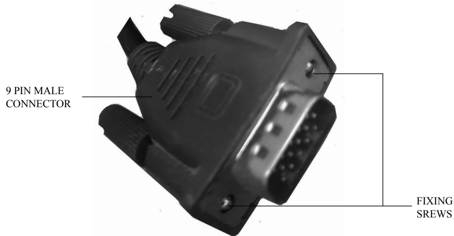
FIG. 4 Inter Connecting Cable
