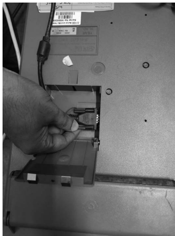
Fig. 20 A Proper insertion of BU cable connector into CU Connector.
