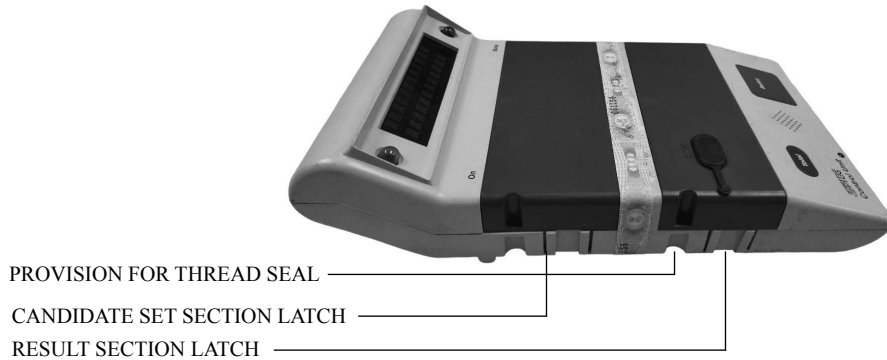
FIG. 7 Front view of Control Unit
